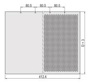
Cover plates perforated version will close the 19" chassis on top and bottom side. The hole diameter is 4 mm, perforation ratio 58 %.
